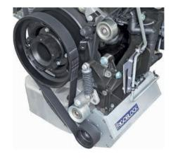
tending to specify the larger size, states regional sales manager Dale Cornes. This unit functions like a simple dynamo: increasing revs increases power output. She adds that this means that the unit increases the truck's idle speed to provide power.
